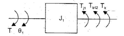
By Newton's second law,  $T_{j1} + T_{b12} + T_k = T$
