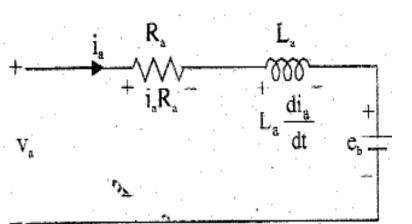
Torque of DC motor is proportional to the product of flux and current. Since flux is constant in this system, the torque is proportional to i<sub>a</sub> alone.
