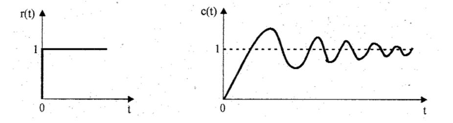
In output response, the system provides oscillations intially and these oscillations are dying with incerease in time. This response is Underdamped System response
