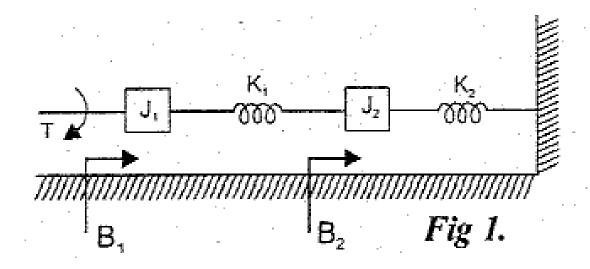
$$J_1 \frac{d\omega_1}{dt} + B_1\omega_1 + K_1 \int (\omega_1 - \omega_2) dt = T$$
