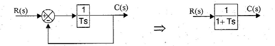
The closed loop transfer function of first order system,  $\frac{C(s)}{R(s)} = \frac{1}{1+Ts}$
