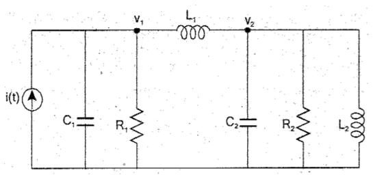
$$C_{1}\frac{dv_{1}}{dt} + \frac{1}{R_{1}}v_{1} + \frac{1}{L_{1}}\int(v_{1} - v_{2})dt = i(t)$$
