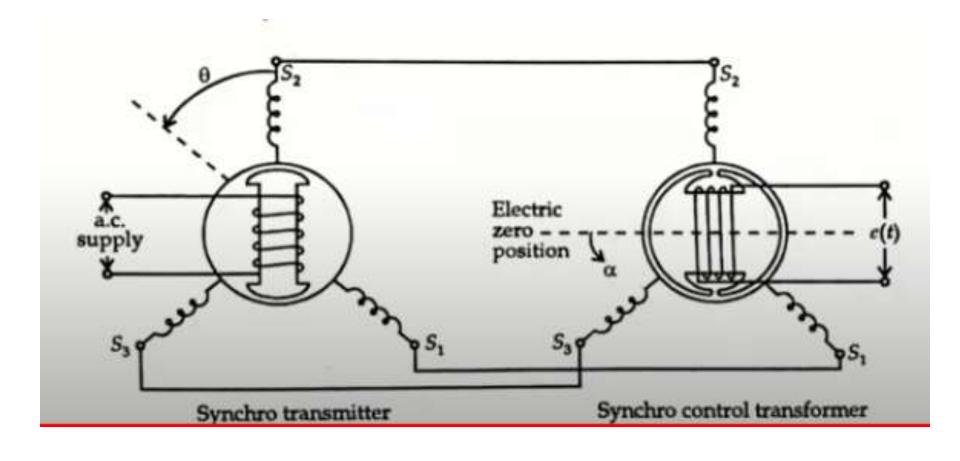
Here e(t) voltage is obtained based on angular position of Rotor
