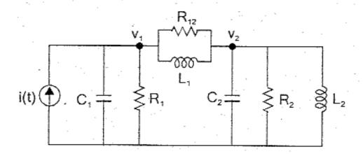
$$C_1 \frac{dv_1}{dt} + \frac{1}{R_1} v_1 + \frac{1}{R_{12}} (v_1 - v_2) + \frac{1}{L_1} J(v_1 - v_2) dt = i(t)$$
