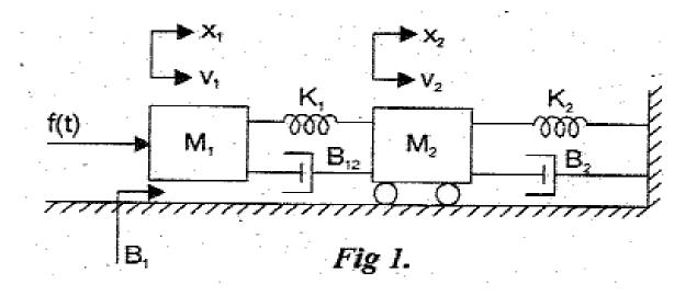
$$M_1 \frac{dv_1}{dt} + B_1v_1 + B_{12}(v_1 - v_2) + K_1 \int (v_1 - v_2) dt = f(t)$$
